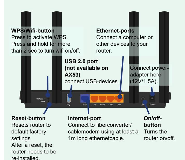
This router can be mounted on a wall or placed on a shelf/desk.
